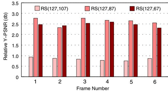
Fig. 13. Relative benefit in decoded PSNR using virtual channels with burst loss at 20% for different FEC used with unreliable virtual channels. Frames of a GoP (ibppbb) in the *Foreman* video sequence are shown.
