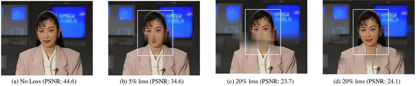
Fig. 5. Shows the impact of burst packet loss on video picture quality for the 3<sup>rd</sup> frame in *akiyo* video sequence. (The grey inner rectangle indicates the region-of-interest in this frame.)
