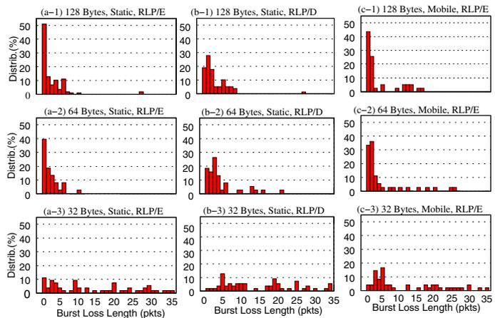
Fig. 11. Sample burst loss distributions for different packet sizes over a commercial CDMA2000 EvDO network. Each experiment consisted of 100000 back-to-back packet UDP samples at 144Kbps. *static* and *mobile* corresponds to stationary and mobile (drive) tests respectively. RLP/E and RLP/D indicates radio link layer as Enabled or Disabled by the client (Samsung SCH/a890).
