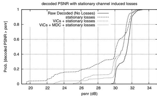
Fig. 15. Cumulative distribution of decoded PSNR for 300 frames in *Foreman* sequence. (stationary channel induced losses)
