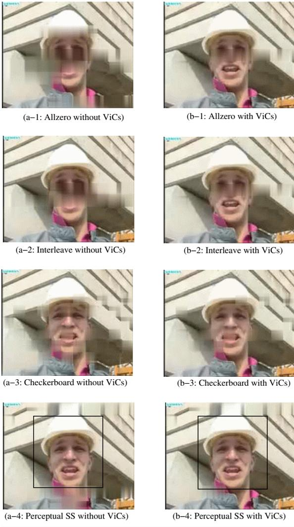
Fig. 19. Shows 55<sup>th</sup> frame of the *Foreman* video sequence using different slice-structured coding schemes. The left half of the figures shows different slice-coding schemes without using virtual channels while right half shows the improvement resulting from use of virtual channels. Figures a-4 and b-4 show visually how perceptual slice-coding improves subjective video quality better than other slice-coding schemes.
