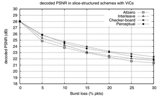
Fig. 18. Impact of burst packet loss (in % slice pkts.) for different slice-structured coding schemes using virtual channels. The vertical axis indicates average luminance PSNR (decoded) for the *Foreman* video sequence.
