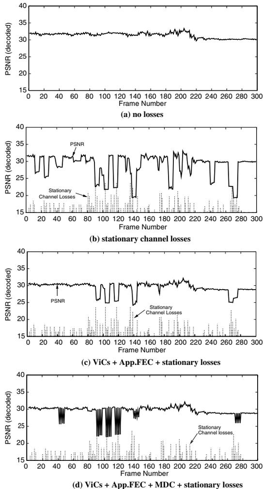
Fig. 14. Decoded PSNR for running 300 frames for *Foreman* video sequence. Shows (top-bottom): (a) decoded PSNR (no losses), (b) decoded PSNR in presence of stationary channel losses, (c) decoded PSNR using 2 virtual channels in presence of stationary losses, and, (d) decoded PSNR using 2 virtual channels with MDC in presence of stationary losses. Also shown are packet errors induced in different video frames (as dotted vertical lines).
