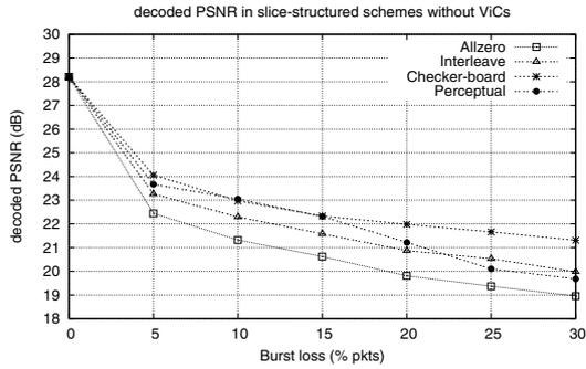
Fig. 17. Impact of burst packet loss (% slice pkts.) for various slice-structured coding schemes without using Virtual channels. The vertical axis indicates average luminance PSNR (decoded) for the *Foreman* video sequence.
