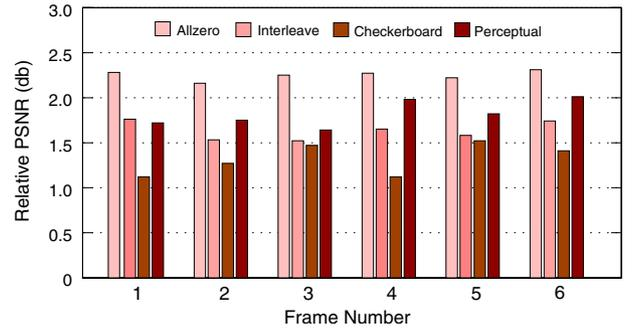
Fig. 20. Relative benefit in PSNR using virtual channels for different slice-based coding schemes at a burst loss of 20%. The different frames correspond to a GoP (ibppb) in the *Foreman* video sequence.
